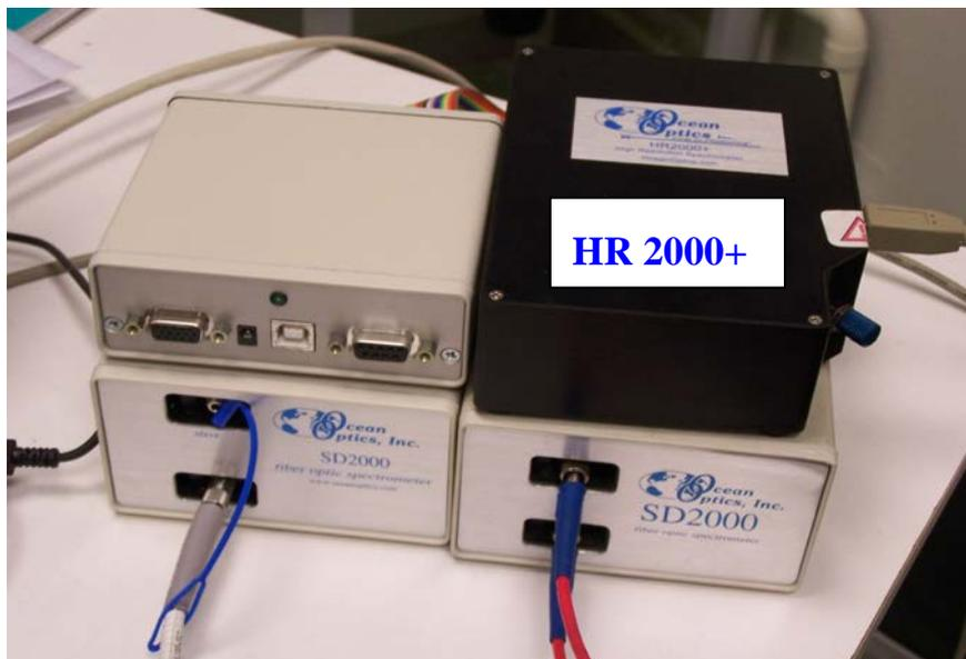
Fig. 6.2 Spectrometer SD 2000 and HR 2000+ used in SLEM system.
