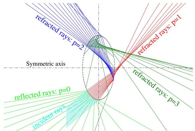
Fig. 1. (Color online) Ray tracing of the first four orders for a spheroid,  $a = 2c$ , of water ( $m = 1.33$ ) illuminated by a plane wave at  $40^\circ$ . For clarity only a portion of the rays is presented.
