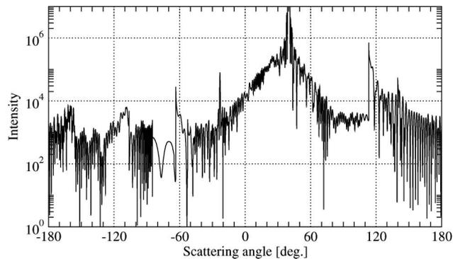
Fig. 3. Scattering diagram of a spheroid ( $a = 2c = 20 \mu\text{m}$ ) of water,  $m = 1.333$ , illuminated by a plane wave of wavelength  $\lambda = 0.6328 \mu\text{m}$  at  $40^\circ$ .
