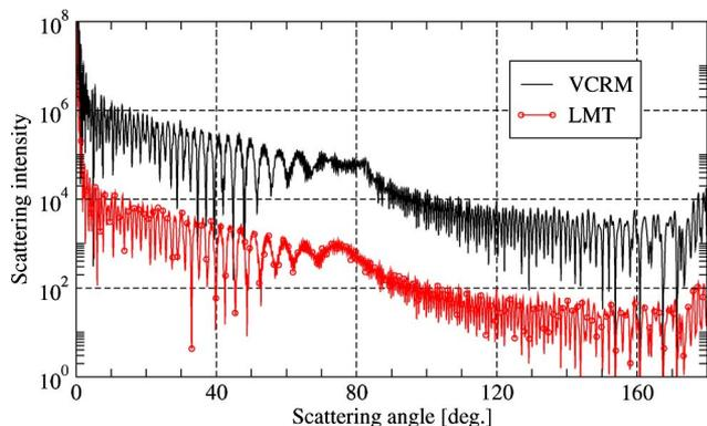
Fig. 2. (Color online) Comparison of scattering diagrams computed by VCRM and LMT for an air bubble in water ( $m = 0.75$ ) of radius  $a = 50 \mu\text{m}$  illuminated by a plane wave of wavelength  $\lambda = 0.6328 \mu\text{m}$ . The result of LMT has been offset by a factor of  $10^{-2}$  for clarity.
